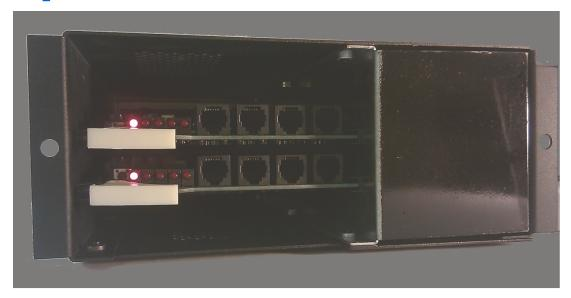
CONVERT DIRECT INWARD DIALING (DID) TRUNKS TO STANDARD ANALOG LINES FOR CONNECTION TO ALL CUSTOMER PREMISE EQUIPMENT (CPE).
